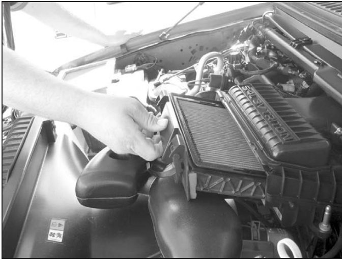
3. Slide the tray with the AIRAID® air filter back into the airbox.
