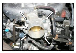
3. Remove the two nuts and two bolts that secure the throttlebody to the intake manifold. Remove the throttlebody and the factory gasket. Remove the two studs that are left in the intake manifold.
