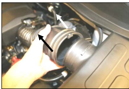
2. Remove the factory intake tube from the air cleaner lid by pushing it towards the engine as shown.
