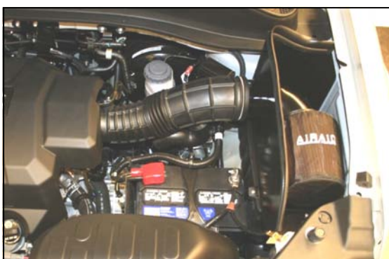
7. Install the supplied weather strip (#3) onto the top of the Quick Fit Panel, starting at the left fender, and working your way towards the front of the vehicle. Slip the Pre-Filter over the Airaid premium Filter.
