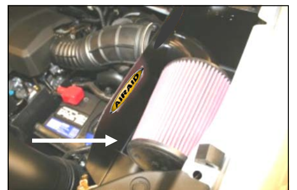
6. Install the Airaid Premium Filter (#1) onto the Quick Fit Panel Tube, and tighten the clamp. Apply the Airaid Foil Decal onto the Panel as shown.
