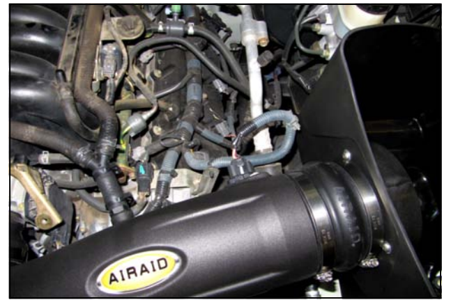
12. Reconnect the factory PCV breathers and spring clamps to the Barbed "Y" Fitting. Reconnect the Mass Air Flow sensor.
