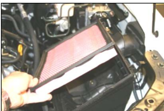
7. Remove the factory air filter.
