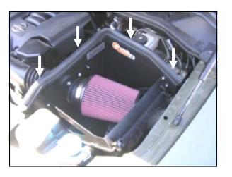
**10.** Install the Airaid Premium Filter (#1) onto the air filter adapter, and tighten the hose clamp. Install the weather strip (#5) onto the Quick Fit Panels as shown (*Note: Start at one corner and work your way around to the end to insure proper alignment of the weather strip).*
