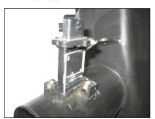
**3.** Using a Phillips head screwdriver, remove two screws and the **MAF** sensor from the factory air box lid. Save the sensor for reuse.
