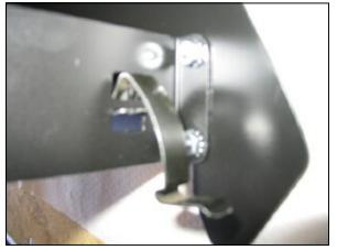
**7.** Remove the clip from the factory air box lid and install it in the Quick Fit Panels as shown.
