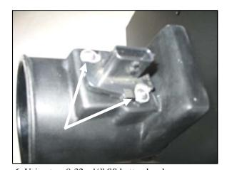
**6.** Using two 8-32 x  $\frac{1}{2}$ " SS button head screws (#11), reinstall the factory **MAF** sensor into the air filter adapter.
