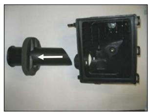
**4.** Remove the factory air box base from the vehicle. Using a flat blade screwdriver, unsnap and remove the factory tube from inside the air box base. Reinstall the factory air box base and the bolts into the vehicle, without the tube.
