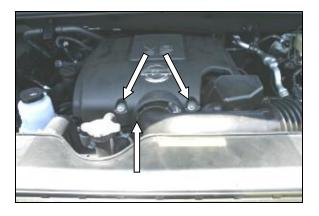
4. Reinstall the factory intake tube, and tighten the hose clamp. Reinstall the engine beauty cover, and tighten the factory bolts.
