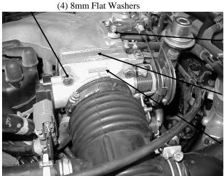
Ref. "D"- (1) Linkage Plate (2) 6mm x 12mm Flat Head Screws
