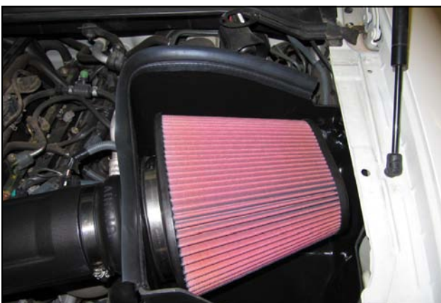
16. Install the Airaid Premium Filter (#1) onto the Filter Adapter then install the Weather Strip (#7) onto the top of the Cold Air Box with the contour rolling away from the Filter.
