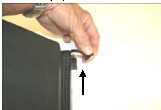
8. Very carefully remove the rear clip from the factory airbox.
