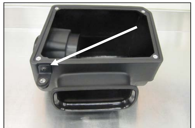
6. Mount the Airbox Bracket as shown, using one 1/4-20 Button Head Screw and a 1/4" Flat Washer. Transfer one factory airbox mounting grommet and steel sleeve from step 3 into the Airbox Bracket.
