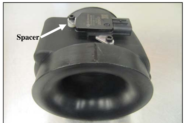
3. Transfer the Mass Air Flow sensor into the Filter Adapter and secure using the two 8-32 Socket Head Screws and Spacers .
