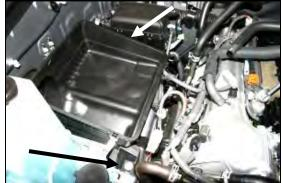
**4.** Using a 10mm socket, loosen the two bolts that hold the airbox base to the fender well, and remove it from the vehicle. There is one bolt on the front of the base, and one bolt at the rear of the base.
