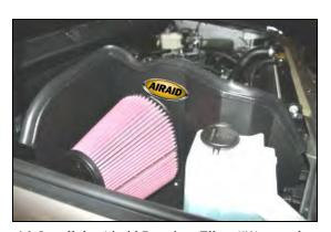
16. Install the Airaid Premium Filter (#1) onto the filter adapter and tighten the clamp. Next install the weather strip (#8) on top of the CAD as shown. For an easier install, start at the fender side of the CAD and work your way towards the radiator. Reinstall the factory beauty cover. Apply the Airaid Decal to the Panel assembly a shown.
