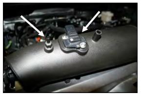
9. Re-install the MAF sensor into the Airaid intake tube (#2) as shown using the supplied 8-32x3/8" button head screws (#12).
