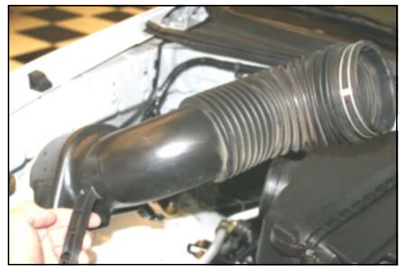
3. Remove the complete intake tube from the vehicle.
