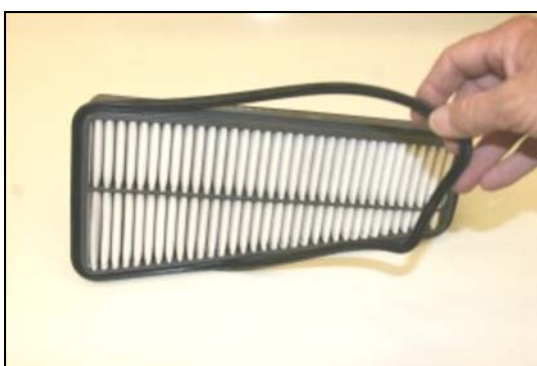
5. Remove the rubber gasket from around the factory air cleaner.
