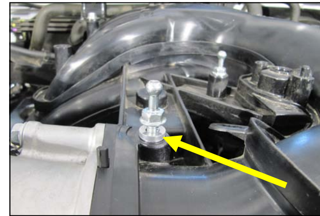
20. Remove the front engine cover mounting post and place the Aluminum Spacer onto the threaded stud like a washer and re tighten.
