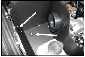
7. Install the CAD assembly into the vehicle. Align the hole in the bottom over the captured nut in the fender well. Install one 16mm hex bolt (#16), and washer (#14). Leave loose for now. Next reinstall the factory bolt removed in step #5, thru the bracket, into the ground anchor in the fender well.
