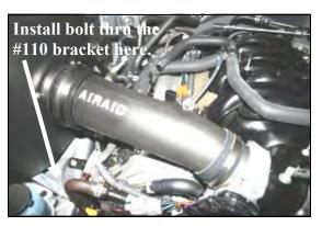
11. Install the Airaid intake tube into the hump hose first, and then into the reducing coupler. Center the tube between the throttlebody, and the CAD, adjust for fit, and then tighten the four hose clamps. Install one 6mmx12mm bolt (#16) and washer (#14) thru the bracket into the captured nut in the fender well.
