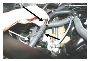
12. Install the 1/2" breather hose (#23) onto the nipple on the Airaid tube. Slide the 1/2" barbed coupler (#21) into the installed breather hose, and secure both ends with the supplied speed clamps (#22).
