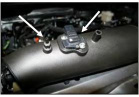
9. Re-install the MAF sensor into the Airaid intake tube (#2) as shown <u>using the supplied 8-32x3/8" button head screws (#12).</u>
