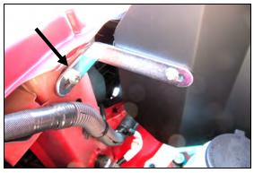
15. Use supplied 10-32 hex head bolt and Fender Washer to secure Panel Bracket. Do not over tighten.
