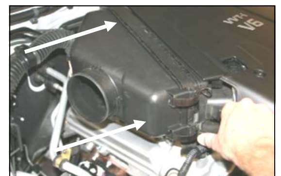
9. Re-install the factory airbox cover, and re-latch both clips.
