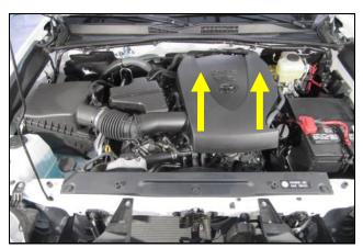
1. Disconnect the negative battery cable. Lift up on the engine cover to unseat it from the mounting grommets, remove it from the vehicle and set aside.
