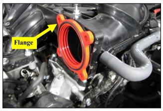
**5.** Insert the PowerAid spacer into the intake manifold as shown. When properly installed, the O Ring flange will be facing outward.
