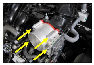
**6.** Reinstall the throttlebody on top of the Poweraid Spacer using the four bolts and washers that are supplied with the kit. Tighten the bolts evenly, in a "X" pattern. Manually cycle the throttle plate by hand and confirm you have full range of motion.
