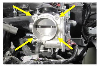
**3.** Remove the four bolts that secure the throttlebody to the intake manifold. Without disconnecting the wiring harness, remove the throttlebody from the intake manifold and set it to the side.
