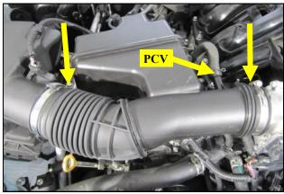
2. Loosen the clamps on the intake tube and disconnect the PCV breather. Remove the intake tube and set it aside.
