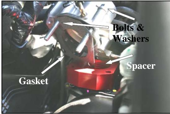
5. With the gasket (#4) on top of the Poweraid Spacer (#1), lift the throttle body up, and slide the spacer between the manifold, and the throttle body. Install four 8mm bolts (#2) and washers (#3) thru the throttle body, gasket, spacer, and into the manifold.
