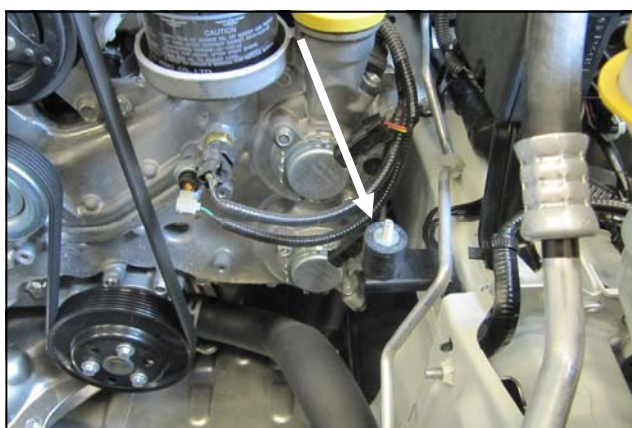
5. Install the CAB Mount into the airbox bracket on the inner fender. Hand tight is sufficient.
