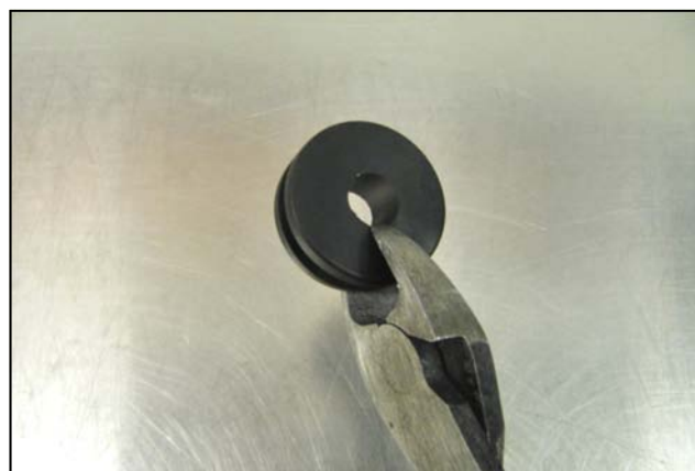
8. Using a pair of diagonal cutters, or similar, split the Harness Grommet.
