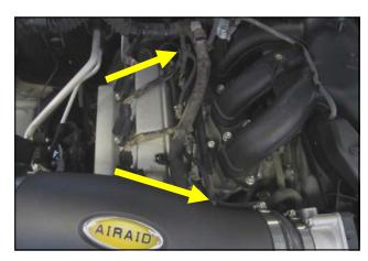
**12.** replace the OEM vacuum line on the fuel pressure regulator with the supplied 20 1/2" 1/8" line. Connect the 1/8" line to the small Fitting on the Intake tube.
