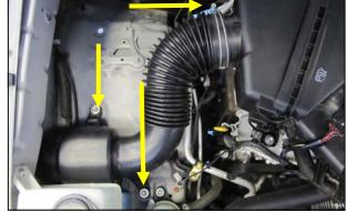
**2.** Loosen the clamp on the factory intake tube and remove the two 8mm bolts securing the other end on the inner fender. Slide the intake tube out from the inner fender hole and set it aside.
