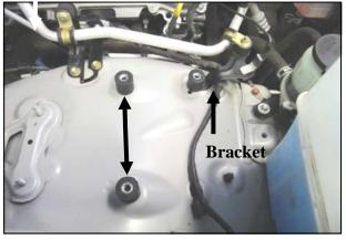
**5.** Install two of the M8 CAB Mounts (#13), hand tight, into the weld nuts on the inner fender as shown. Use the third CAB Mount to replace the 8mm bolt holding the A/C bracket.
