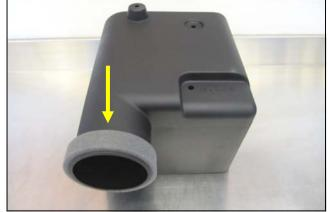
**6.** Apply the self adhesive, Foam Weatherstrip (#9) onto the air inlet on the Cold Air Box (#3).
