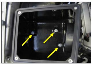
**7.** Mount the Cold Air Box onto the CAB Mounts using the three 8mm Bolts (#14) and 5/16 Flat Washers (#15)
