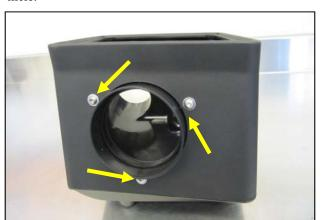
**7.** Mount the Filter Adapter (#5) to the Cold Air Box, as shown, using three  $1/4-20 \times 1/2$ " Button head Bolts (#16) and 1/4" Flat Washers (#17).
