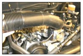
**12.** Remove the factory intake tube.
