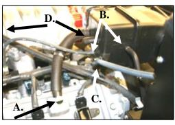
11. A) Disconnect breather hose at the valve cover. B) Disconnect 1/4" and 1/8" vacuum lines on the back of the factory intake tube. C) Unclip MAF wire harness retainer from the intake tube. D) 01-03 Sequoias and 00-02 Tundras only; remove 3/8" vacuum hose between factory intake tube and metal fitting on top of the intake manifold. (Hose Not Shown)
