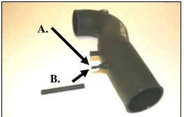
14. A) Install the 1/4"Barb x 1/8"NPT fitting (#14) into the Airaid Modular Intake Tube (MIT) (#5).
