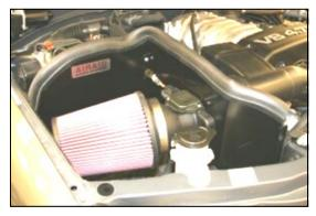
**8.** Install the Airaid Premium Filter (#1) onto the **MAF** adapter. Next install the weather strip (#10) on top of the **CAD**. Start at the radiator end and work you way towards the back.
