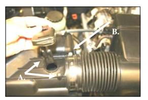
1. Stage I Disconnect the negative battery cable! A) Remove the two screws, and remove the Mass Air Flow (MAF) sensor from the factory airbox. Leave the wiring harness connected, and set it aside. B) Loosen the hose clamp on the intake tube
