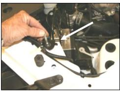
**6.** With a 10mm socket, remove and save the bolt from the anti-lock brake bracket. It will be reinstalled later in step #9.
