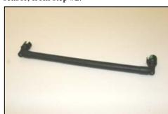
**17.** Install the 3/8"x12" hose (#7) onto the factory breather ends as shown.
