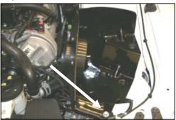
**8.** Place the **CAD** into the inner fender, align the bolt holes and re-install the bolt from step #6.
