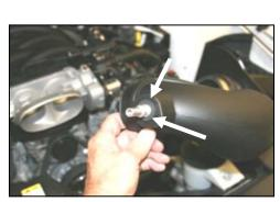
**11.** Install the supplied grommet (#13) and aluminum fitting (#16) into the Airaid intake tube as shown.
