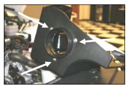
7. <u>Install the air filter</u> adapter (#5) into the Cool Air Dam (#7) as shown, using 3 button head bolts (#9) and ½" flat washers (#10).
