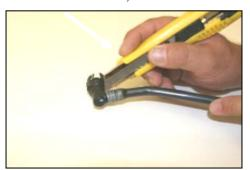
**16.** <u>VERY CAREFULLY</u> ! Using a razor blade, cut the plastic tube off both of the factory breather hose ends as shown.
