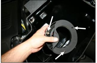
4. A.) Using an 8mm socket, remove the two factory 5. Remove the factory air box assembly from the vehicle. 6. Prepare the Filter Adapter for installation by positioning the Adapter Gasket on the mounting side and lining up the holes.
