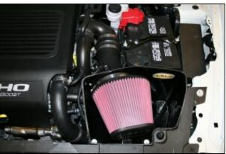
11. A.) Place the CAB in the original location of the 12.Install the Airaid Premium Filter onto the Filter adapt-
