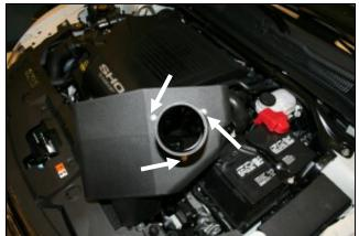
Box, CAB using the three 1/4"-20 hex head bolts and 1/4" flat washers as shown.
