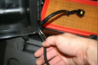
2.A.) Unfasten the factory air box clips and separate 3. Using a pair of needle nose pillars, carefully compress the fins of the wiring harness anchor and pull it out of the air box lid.
