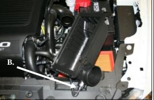
the upper half of the air box from the intake assembly. **B.**) Disconnect the air temperature sensor.
