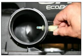
7. Install the Filter Adapter to the inside of the Cool Air 8. A) Install the Hump Hose, large side first onto the 9. Remove the Air Temperature Sensor from the factory air box by rotating the sensor 1/4 turn counter clockwise and pulling outward.
