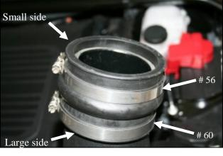
**CAB** tube. Loosely install the #56 Hose Clamp on the small side of the Hump Hose, and the #60 Hose Clamp 1) on the Large side. (B) Slide the Hump Hose and Clamps downward on the tube, creating a compact assembly as shown.
