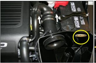
Factory Air box and secure using the factory hardware er and tighten the clamp. from step 4. B.) Slide the coupler and clamps onto 90 deg. Elbow pipe and tighten the clamps. C.) Reconnect the Air Temperature Sensor. Apply the Airaid Decal inside of the Airbox as shown.
