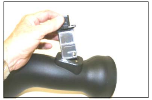
12. Install the MAF sensor from step #5 into the Airaid Intake Tube. Use the two supplied 8-32 button head bolts (#10), to securely fasten the MAF sensor. Do Not Use The Factory Screws!
