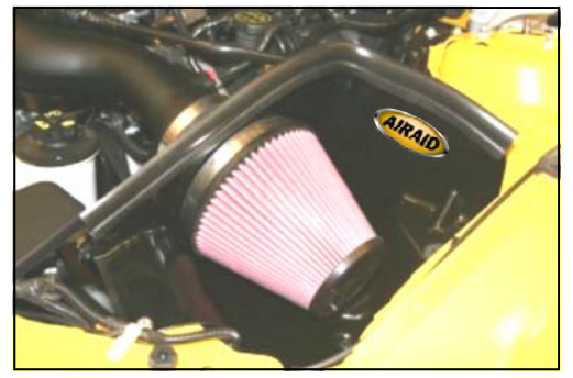
15. Install the Airaid Premium Filter (#1) onto the filter adapter (#5). Next install the weather strip (#7) on the top of the CAD as shown. Start at the front of the CAD and work towards the rear. Apply the Airaid Decal inside the CAB as shown.
