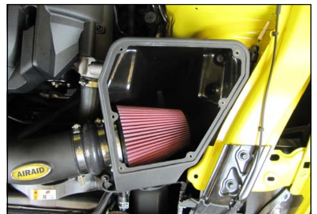
18. Install the Airaid Premium Filter onto the Filter Adapter inside of the Airbox.
