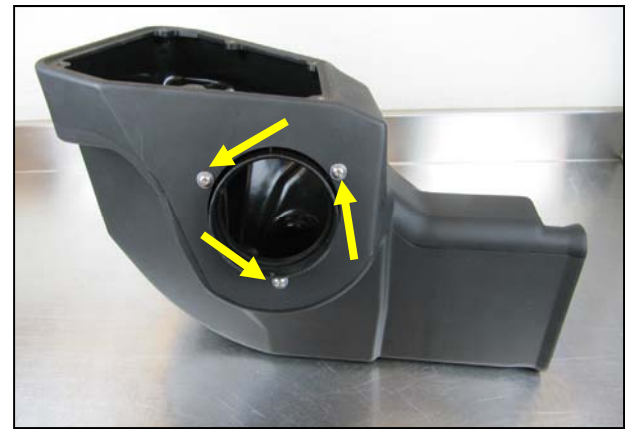
12. Install the Filter Adapter onto the Cold Air Box as shown using the three 1/4-20 Button Head Screws and 1/4" Flat Washers.
