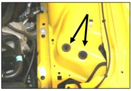
**4.** Make sure that you retain the factory grommets in the inner fender from the bottom of the factory airbox.
