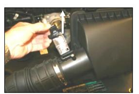
**5.** Using the supplied #20 torx bit, remove 2 factory screws, and remove the MAF sensor from the factory tube. (Save the MAF sensor for reinstallation in step #12).
