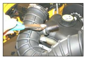
**6.** With a pair of side cutters, remove the metal band that holds the plastic breather fitting in the factory tube. Next remove the fitting from the tube, and save it for reinstallation in step #11.
