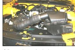
**3.** Remove the complete intake system as an assembly.
