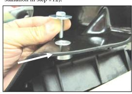
**8.** Slide the Aluminum Spacer (#17) underneath the **CAD** and into the hole as shown. Secure the CAD to the inner fender using the OEM bolt from step # 2 and the supplied 1/4" Fender Washer (#18).
