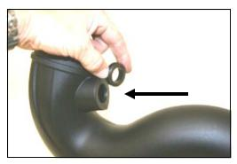
**10.** Install the supplied grommet (#16), into the Airaid Intake Tube (#2)
