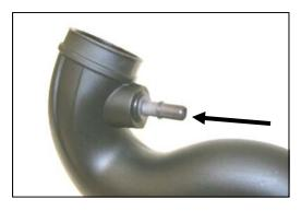
**11.** Install the factory fitting from step #7 into the grommet (#16) from step #10.
