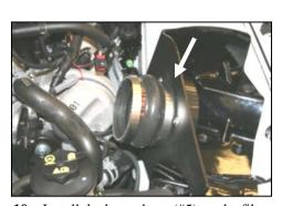
**10.** Install the hump hose (#5) on the filter adapter (#6), with two #72 hose clamps (#13). Tighten <u>only</u> the clamp next to the **CAD**.
