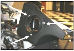
7. Install the air filter adapter (#6) into the Cool Air Dam (#7) as shown, using 3 button head bolts (#9) and 1/4" flat washers (#10).
