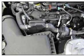
6. Release the one-time use clamp that secures the sound tube to the drum and then disconnect and remove the sound tube from the vehicle.
