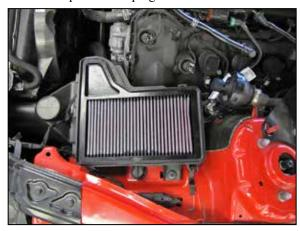
8. Release the clips the secure the upper air filter housing and then remove the factory air filter. Install the AIRAID® replacement air filter and resecure the upper housing with the factory clips.
