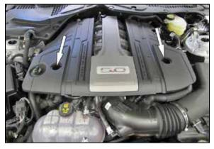
3. Remove the two nuts that secure the decorative engine cover and remove the cover from the engine.
