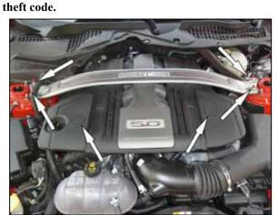
2. Remove the four nuts that secure the strut brace and then remove the strut brace from the vehicle. Pop up the two-round bolt covers.
