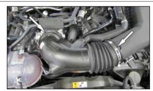
5. Loosen the hose clamps that secure the intake tube to the air filter housing and throttle body and then remove the intake tube from the vehicle.
