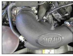
12. Install the AIRAID® intake tube assembly into the coupler hoses, adjust for best fit and then secure with the provided hose clamps. Connect the factory vent lines to the fittings installed into the intake tube.
