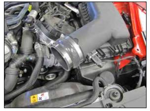
10. Install the provided coupler hose onto the air filter housing and secure with the provided hardware.
