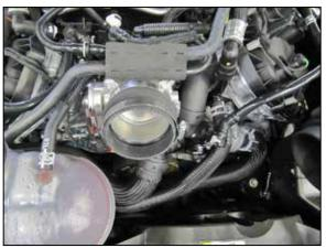
9. Install the provided coupler onto the throttle body and secure with the provided hose clamp.
