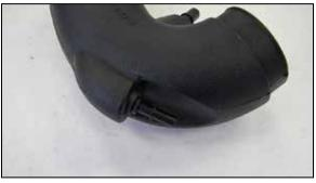
11. Install the provided vent fittings into the AIRAID® intake tube as shown.
