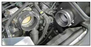
16. Install the provided hump coupler onto the throttle body and straight coupler onto the filter adapter and then secure with the hose clamps provided.
