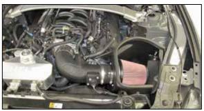
**20. Double check your work!** Make sure there is no foreign material in the intake path. Make sure all clamps, hoses, bolts, and screws are tight. Double check the hood clearance! **Reconnect the negative battery cable!**
