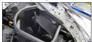
12. Reinstall the factory foam air dam.
