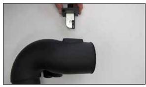
14. Install the mass air sensor assembly into the AIRAID<sup>®</sup> intake and secure with the provided hardware.
