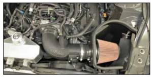
19. Connect the factory vent lines to the fittings installed into the AIRAID<sup>®</sup> intake tube.
