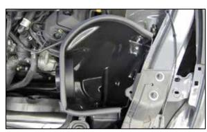
11. Install the AIRAID<sup>®</sup> filter housing assembly into the vehicle and secure with the factory bolt used to secure the factory housing.
