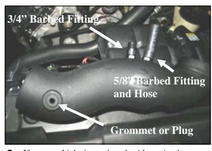
**4.** Remove the two factory grommets from the bottom
