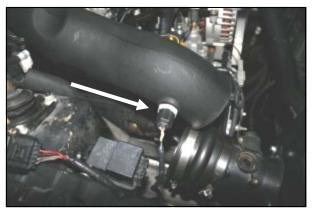
11. On 1999-01 Models, Carefully install the factory intake temp sensor into the grommet in the Airaid Intake Tube.
