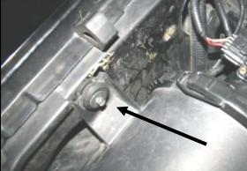
**3.** Remove the bolt that holds the factory air filter canister to the inner fender. Next remove the factory air intake tube from the throttlebody, and then the MAF housing. Now with a twisting motion re-
