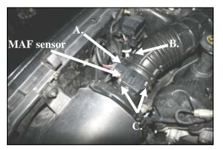
2. A.) Loosen the factory intake tube hose clamp on the Mass Air Flow (MAF) sensor housing. B.) Carefully remove the intake air temperature sensor from the factory intake tube(1999-01 models). C.) Using the supplied T-20 torx bit, remove two screws, and remove the MAF sensor from the MAF housing. Set the temp sensor and MAF sensor to the side for reinstallation later.
