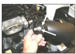
**11.** Install the supplied grommet (#14) and aluminum fitting (#17) into the Airaid intake tube as shown.
