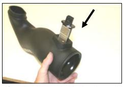
13. Align the two slots in the tubes, and install the factory mass air sensor removed from step #5. Make sure the screw holes line up, then install the two supplied button head screws. (#13). **DO NOT USE THE FACTORY SCREWS!!**
