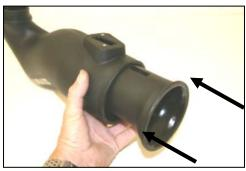
**12.** Install the Modular Venturi Tube (MVT) (#3) into the Airaid Intake Tube (#2) as shown. **(SEE #22 BELOW!!)**
