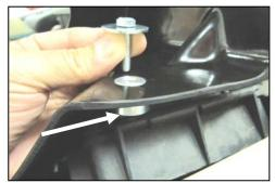
**9.** Slide the Aluminum Spacer (#14) underneath the **CAD** and into the hole as shown. Secure the CAD to the inner fender using the OEM bolt from step #3 and the supplied 1/4" Fender Washer (#15).
