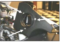
7. <u>Install the air filter</u> adapter (#6) into the Cool Air Dam (#7) as shown, using 3 button head bolts (#9) and ½" flat washers (#10).
