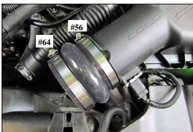
7. Slide the Hump Hose, one #56 Clamp, and one #64 Clamp onto the air box outlet as shown. Do not tighten the Clamps at this time.
