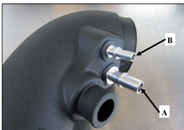
5. Install the Grommets and Fittings into the Modular Intake Tube. A) All models will require the use of the 5/8" Fitting and the 5/8" Grommet. B) Automatic transmission equipped vehicles will also use the 3/8" Fitting and 3/8" Grommet.
