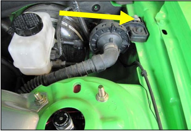
13. Remove the entire Resonator tube assembly and all associated stand offs from the intake tube and the vehicle. Remove the 6mm bolt securing the diaphragm housing to the inner fender remove the tubing from the Fire wall.
