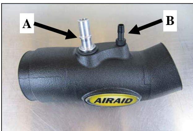
4. Install the Grommet and Fittings into the Modular Intake Tube as shown. A) All models will require the use of the 5/8" Fitting and the 5/8" Grommet. B) Automatic transmission equipped vehicles will also use the Barbed Fitting. Apply the Airaid Decal as shown.
