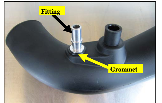
7. Insert the Grommet and Aluminum Fitting into the Airaid Intake tube as shown.
