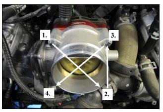
**4.** Insert the provided bolts with washers through the throttlebody, gasket, and Poweraid Spacer and tighten them in an "X" Pattern.
