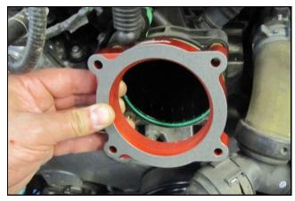
**3.** Install the Poweraid Spacer between the throttlebody and the intake manifold with the supplied gasket next to the throttlebody as shown. Make sure the "flow" arrow that is printed on the spacer is pointing towards the intake manifold.
