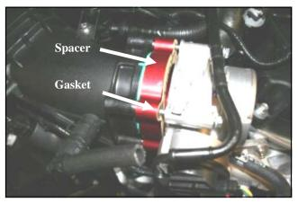
**4.** Position the Poweraid Spacer between the throttlebody and the intake manifold with the supplied gasket next to the throttlebody as shown. Make sure the "flow" arrow that is printed on the spacer is pointing towards the intake manifold. Insert the provided bolts and washers through the throttlebody, gasket, and Poweraid Spacer.
