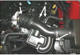
1. <u>Disconnect the negative battery cable!</u> A.) Disconnect the breather line or lines, from the Factory intake tube.
