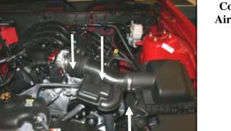
7. Reinstall the intake tube, tighten the two hose clamps, and reconnect the breather line or lines. **Re-connect the negative battery cable!**  Contact your nearest Airaid dealer for an Airaid Intake System for your car, truck or SUV.
