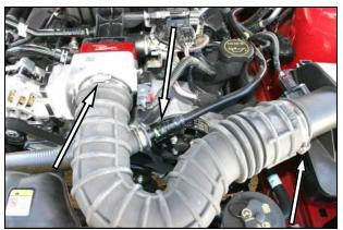
4. Reinstall the intake tube, and tighten the hose clamps. Reconnect the breather hose to the intake tube.
