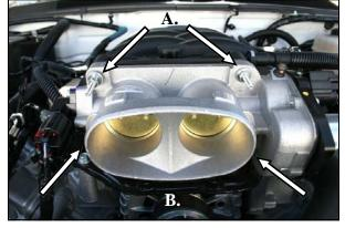
1. **Disconnect the negative battery cable!** Using a 5/16" socket, loosen two hose clamps that hold the intake tube between the throttle body, and the air cleaner lid.
