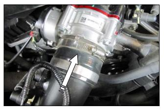
**4.** Slide the throttle body inlet tube back onto the throttle body and tighten the clamp.
