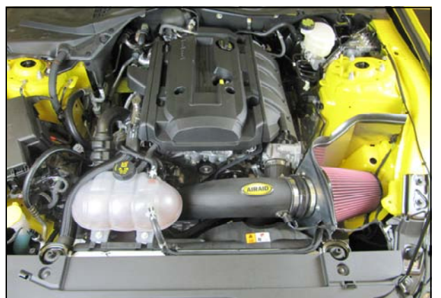
24. Double check your work. Make sure all clamps, hoses, bolts, and screws are tight. Double check the hood clearance. Reconnect the negative battery cable.
