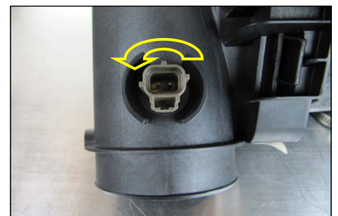
9. Tilt the air temp sensor rearward so the locking tab clears the ramp and rotate it counterclockwise 1/4 turn to release it.
