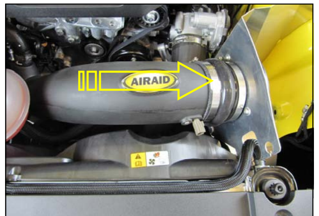
21. Slide the Airaid Intake Tube into the Hump Hose and tighten all four Hose Clamps. Apply the Airaid Bubble Decal onto the Intake Tube as shown.
