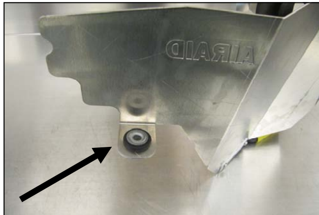
14. Transfer the OEM air box grommet and anti-crush sleeve into the Panel assembly as shown.
