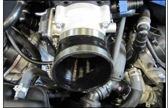
**10.** Install the Silicone Reducer (#6) and Hose clamps onto the throttle body. Place the #56 clamp (#15) on the Throttle body side of the reducer, and the #64 clamp (#14) on to the tube side.
