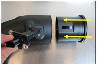
intake tube using two provided 8-32x3/8" screws (#12). Do Not Use The Factory Screws!
