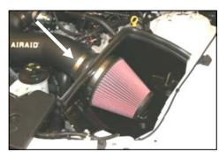
**15.** <u>Install the Airaid Premium Filter</u> (#1) onto the filter adapter, and tighten the clamp. Install the weather strip (#8) on the top of the **CAD** as shown
