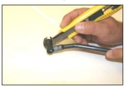
**16.** <u>VERY CAREFULLY</u> ! Using a razor blade, cut the plastic tube off both of the factory breather hose ends as shown.
