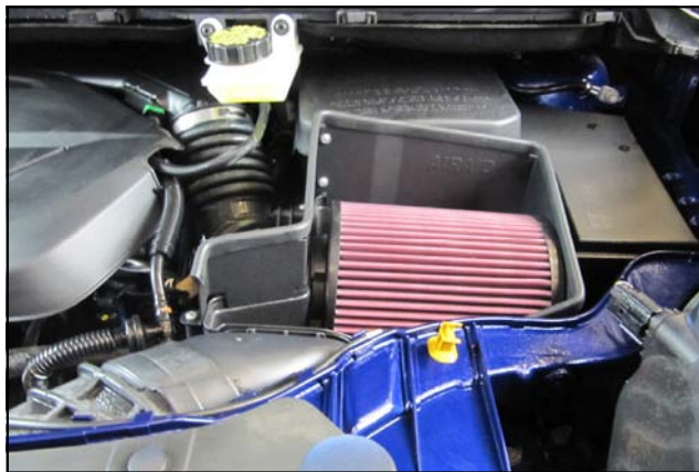
14. Install the Edge Trim (#4) onto the top edge of the Panel assembly.
