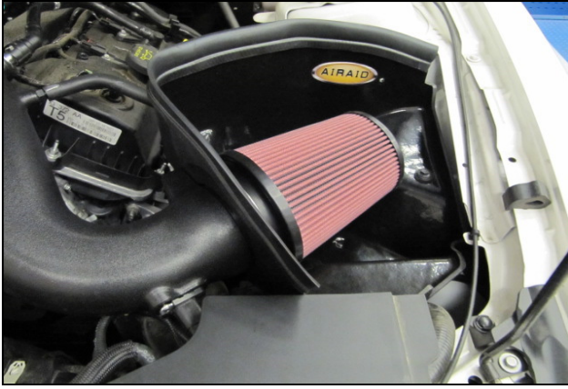
13. Install the Weather Strip (#5) onto the CAB starting at one end and working your way around.
