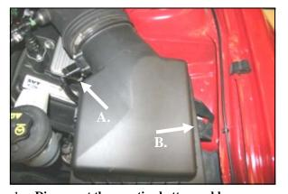
1. **Disconnect the negative battery cable.** A.) Slide out the RED locking tab on the bottom of the Mass Air Flow sensor (MAF) connector, and then squeeze the BLACK tab and disconnect the connector from the sensor. B.) Using a 10mm socket, remove and save the bolt that holds the air filter box to the inner fender. It will be reinstalled in step #13.
