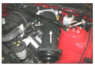
**11.** Install the Airaid Intake Tube into the oval hump hose. For ease of installation, don't tighten the clamps yet!
