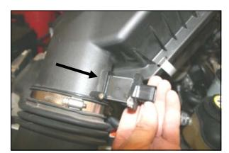
**5.** Using the provided #20 torx bit, remove two factory screws and the Mass Air Flow sensor from the fac-
