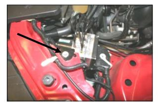
**6.** Using a 10mm socket, remove and save the bolt from the top of the anti-lock brake bracket. It will be
