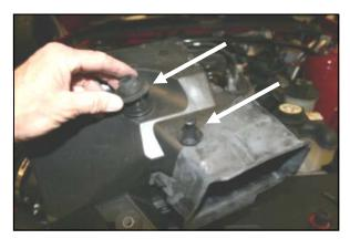
**4.** Remove the two factory grommets from the bottom of the factory airbox and replace them back into
