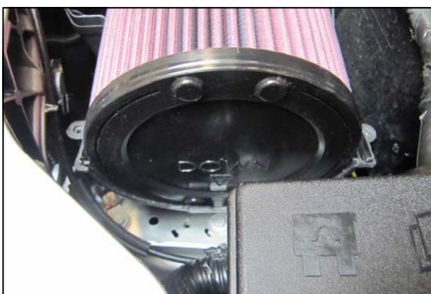
7. Install The Airaid Premium Filter and clamp into the air box as shown, with the Arrow pointing Down and the Lugs in the correct position. When properly installed, the Filter top will be completely inside of the airbox lower half.
