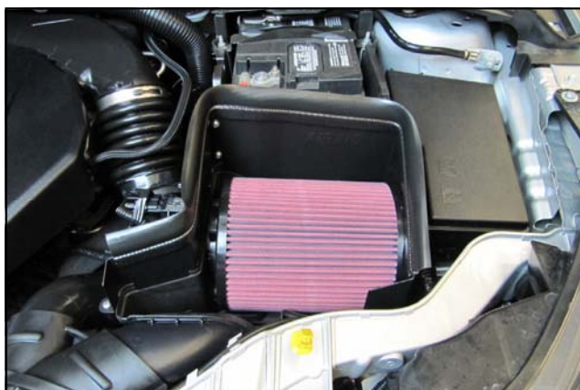
14. Install the Weather Strip onto the Panel assembly with the contour rolling away from the Air Filter.
