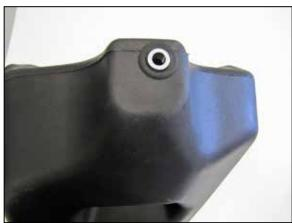
8. Install the provided grommet and spacer into the AIRAID® air filter housing as shown.
