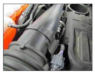
3. Disconnect the mass air wiring harness clip from the intake tube.
