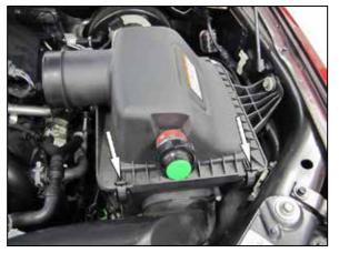
5. Release the two clips that retain the factory upper air filter housing and then remove the upper housing from the vehicle.
