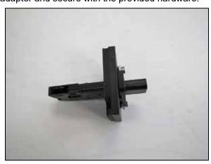
13. Install the provided gasket onto the mass air sensor adapter. Remove the mass air sensor from the factory housing and then install it into the AIRAID® adapter and secure with the provided hardware.
