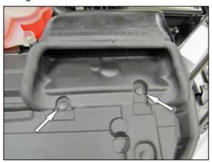
6. Remove the two clips that secure the fresh air intake duct to the core support.
