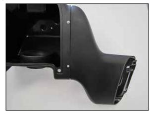
10. Install the AIRAID® fresh air intake duct into the air filter housing and secure with the provided hardware.
