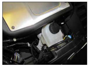
20. Connect the two wiring harness clips to the  $\mathsf{AIRAID}^{\texttt{®}}$  air filter housing.
