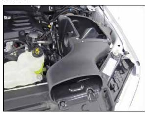
11. Install the AIRAID® air filter housing assembly into the vehicle and secure with the provided hardware.
