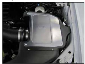
17. Install the AIRAID® air filter onto the adapter and secure with the provided hose clamp and then install the air filter housing lid and secure with the provided hardware.
