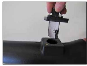
14. Install the mass air sensor adapter into the AIRAID intake tube and secure with the provided hardware.
