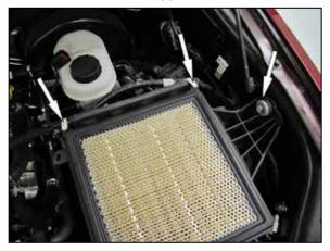
7. Disconnect the mass air sensor wiring harness from the lower air filter housing. Remove the bolt that secures the lower air filter housing to the inner fender and then remove the lower housing from the vehicle
