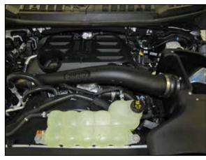
15. Install the AIRAID® intake tube into the factory turbo inlet coupler and the coupler at the filter adapter, adjust the tube for best fit and then secure with the provided hose clamps.
