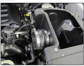
12. Install the provided hump coupler onto the filter adapter and secure with the provided hardware.
