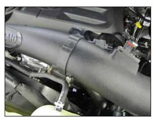
19. Secure the mass air sensor wiring clip to the intake tube.
