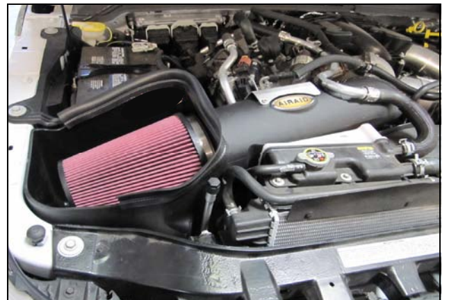
18. Install the Airaid Premium Filter inside the CAB and complete the install by trimming the CAB with the Weather Strip.
