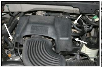
Disconnect the negative battery cable. Using a 10mm socket, remove the three bolts that secure the beauty cover over the throttlebody. Remove the cover and save these parts for reinstallation in step #16.
