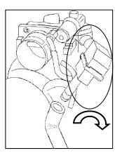
**15.** <u>4.6L engines</u>: Rotate the resonator box 90 degrees to provide clearance for the 3/4 x 12" L-hose (#7). Install the 3/4"x12" L-hose (#10) onto the Airaid Intake tube and the resonator box and secure it using the two #22 speed clamps (#23).
