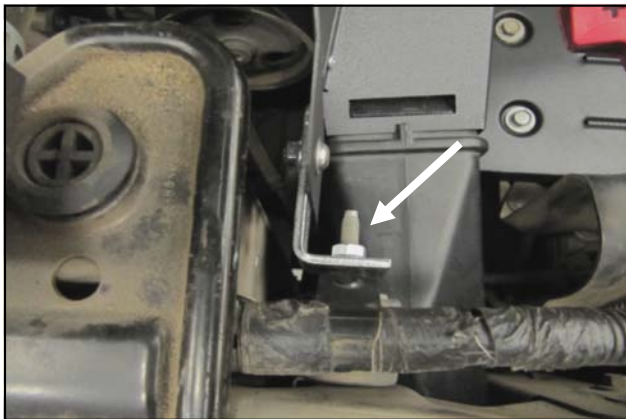
13 . Place the second bracket 140 (#12) onto the 6mm core support stud and secure using the 6mm flanged nut (#18). Attach the Bracket to the Panel using one 1/4-20 Button Head Bolt, 1/4" Flat Washer, and 1/4-20 Flange Nut.
