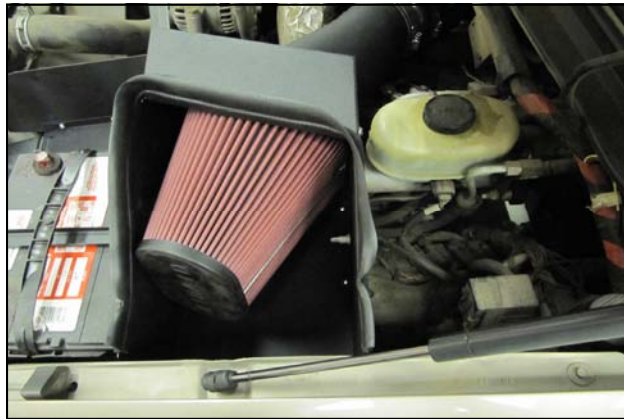
17. Install the CAD Lid (#6) as shown and secure using four 1/4-20 Button Head Bolts and 1/4" Flat washers. Complete the Installation by attaching the Weather Strip (#9) to the CAD assembly edge surrounding the Filter.
