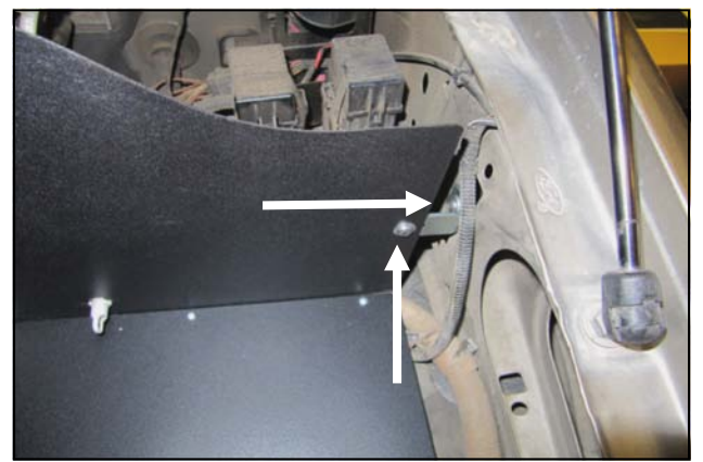
12. Vehicles equipped with a power distribution box mounted on the left inner fender, will remove the bolt from the factory bracket, slide in the bracket 140 (#12) and replace the factory bolt. If you don't have the distribution box, install the provided 1/4-20 button head bolt (#14), washer (#15), and nut (#16), through the inner fender, and tighten. Now tighten the button head bolt that holds the L-bracket to the panel.
