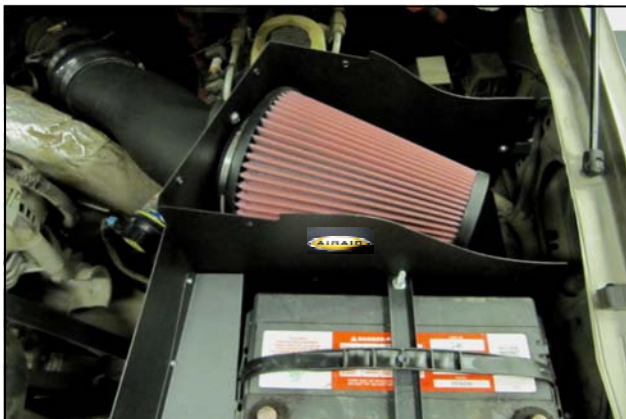
16. Install The Airaid Premium Filter and apply the Airaid Decal as shown.
